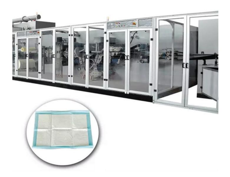
Underpad production line with different type: 3 Layer Underpad, 5 Layer Underpad
